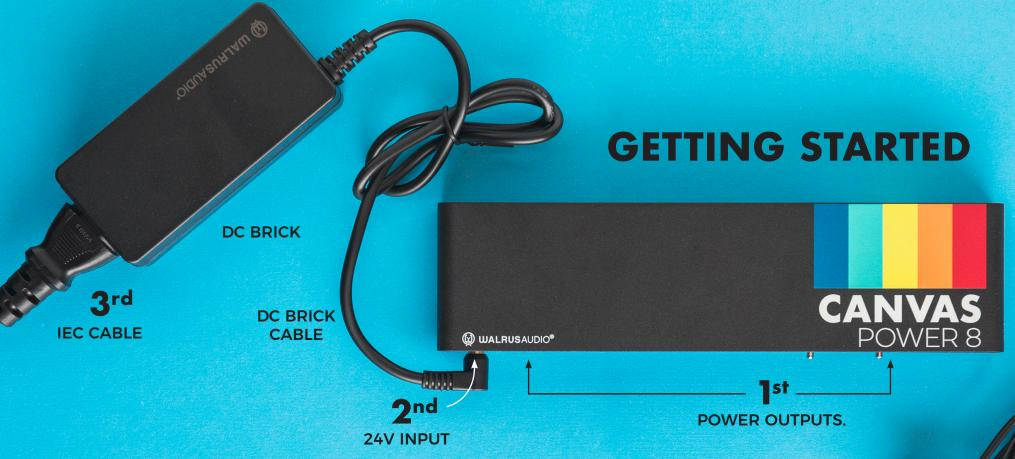
First, wire up your board. Connect your pedals to the appropriate power outputs. Second, connect the DC Brick cable to the 24V DC Input. Finally, connect the IEC cable to the DC Brick to power your pedals.
