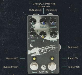
\*The use of an isolated power supply is recommended for powering all Walrus Audio
