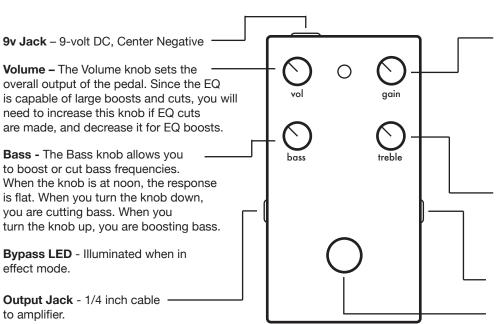
Gain – The Gain knob on the 385 is similar to the volume knob on the Bell & Howell amp. The amp does not have a master volume - only a single volume knob that controls the gain in the pre-amp section of the projector, which sets how dirty and responsive the amp will be. Run the 385 Gain knob low for warm clean tones, that will still break up when hit hard, mid way for responsive grit, or high for huge walls of drive, just like the amp.
