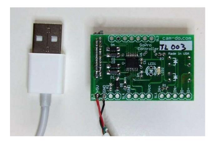
Power is not required for the controller board. This connection is identical to connecting a USB charger to the mini-USB jack on the side of the camera. The short USB cable will fit through the slots in the GoPro extended skeleton back door or can be coiled inside the fully waterproof extended back door when not needed.
