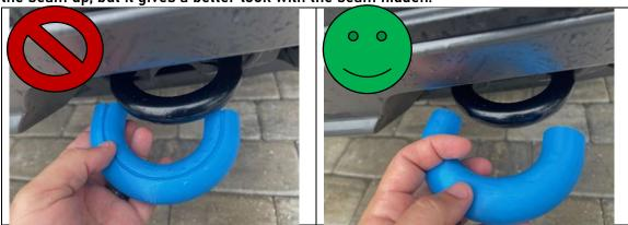
2. Open the seam on either end, and slide over that same side of the tow hook.
