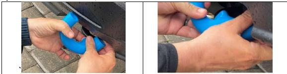
3. Once you have that side around the hook, carefully run your finger along the seam to work it over the rounded part of the tow hook.
