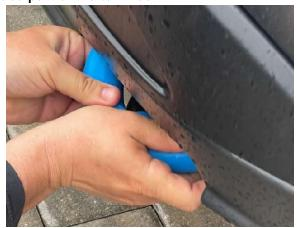
4. The hard part is done, finish positioning the opposite side so that it properly wraps around the hook.
