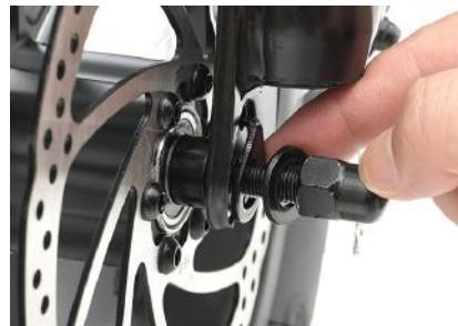
27 Tighten the nuts on both sides of the bearing
