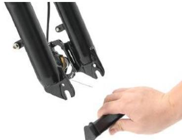
25 Align the brake rotor with the brake pads
