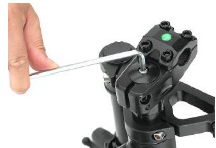
7 Loosen the four stem bolts on the head tube
