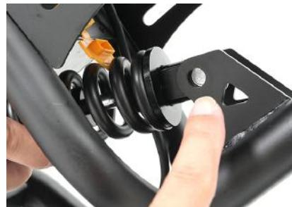
34 Insert the screw into the mounting hole
