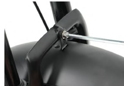
31 Tighten the left and right screws to secure both fender brackets
