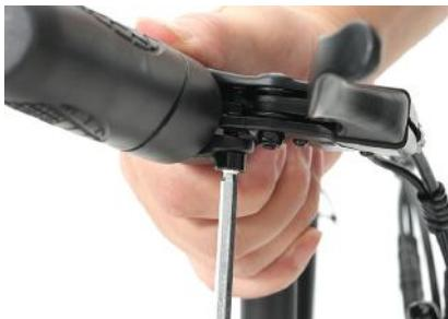
14 Release the front light clamp and align both sides to the same height
