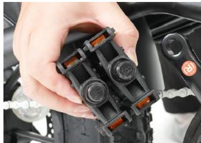
39 Turn the right pedal clockwise and the left pedal counter-clockwise, then tighten with a tool
