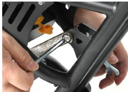
33 Extract the rear shock absorber and align its mounting points with the frame holes
