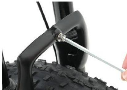
29 Align the fender mounting holes with the fork brace holes
