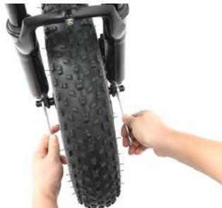
28 Remove the center screw from the fork brace
