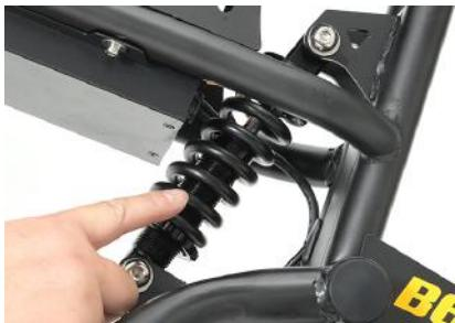
35 Tighten the nuts on the shock absorber
