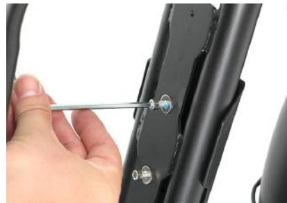
37 Install the water bottle cage and tighten the screws
