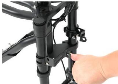
15 Remove the two side screws from the headlight housing
