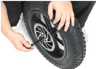
23 Remove the plastic protective shim from the front brake
