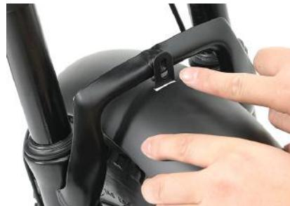
30 Tighten the screws to secure the fender to the fork brace
