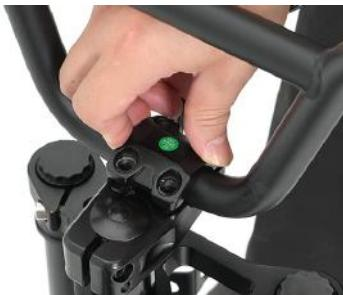
12 Tighten the four bolts on the headset retainer with a tool
