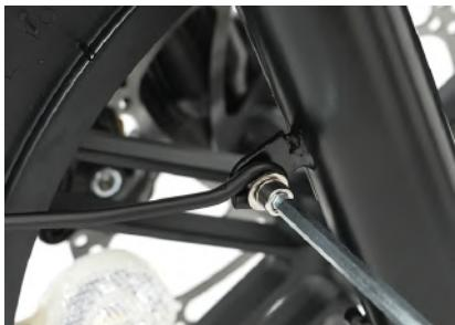
32 Remove screws from the metal guard bar and uninstall the guard bar
