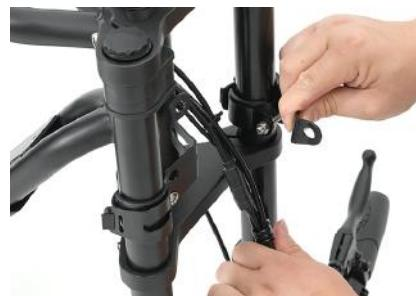
10 Insert the steerer tube into the head tube recess
