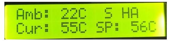
10. You have 30 seconds to complete setup, "S" will change to "x" or "w" when time runs out, at which time you can repeat step 8 above to re-enter setup mode if necessary.
