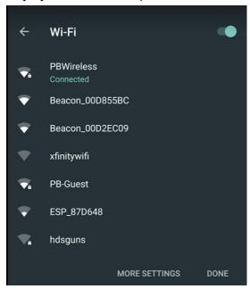
13. If a configuration page does not open automatically after connecting, open a browser on the device that is connected to the Beacon\_xxxxxxxx access point, a page should load automatically, if the page does not load automatically enter 192.168.4.1 in the address bar and press enter.
