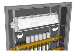
Position the basis slightly tilted onto the DIN rail and latch it in.
