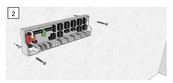
Mark the two fixing holes for the basis and drill them. The basis must horizontally align. Install the basis with dowels and screws (2 units M4) depending on the condition of the wall.
