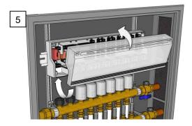
Close the cover and apply mains voltage. Now the basis is ready to operate.
