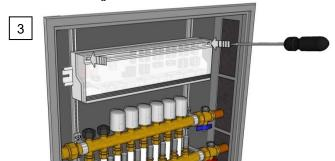
Loosen the casing cover at both latching points with a screwdriver and remove it.
