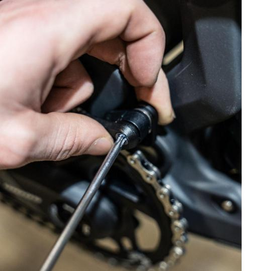
**Step 8**Using your T25 Torx, tighten to 2.5Nm.
