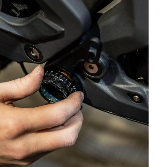
Re-install the drive side bottom bracket cup, torque to 50Nm. Add grease/ anti-seize if needed.
