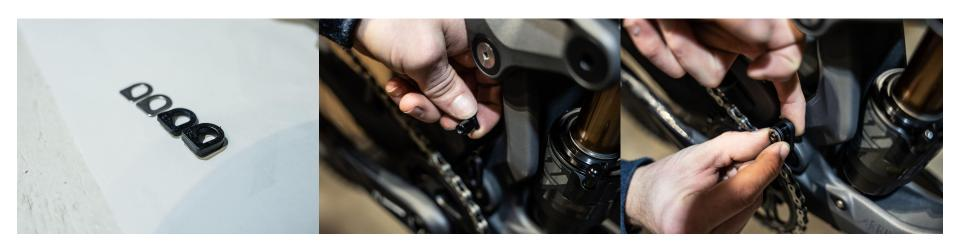
Install the guide block using 1  $\times$  2mm plastic and 1  $\times$  1mm metal spacers.
