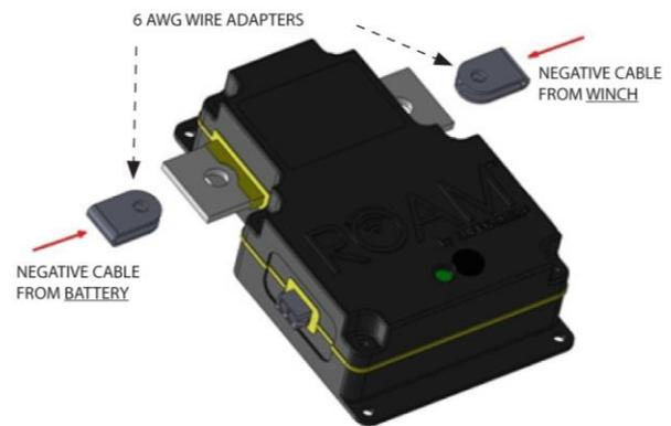
For winches with 6 AWG or smaller power cables, such as TERRA ATV winches, use supplied wiring Adapters. Slide adapters onto ROAM™ unit connections points, and use supplied hardware for connecting power cables. Attach winch negative battery cable to right side of ROAM™ unit. Connect supplied negative battery cable to left side of ROAM unit, and connect to Battery Negative.
