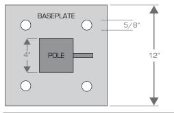
The diagram above is a top-down view of a 1/2" thick baseplate and pole assembly showing plate and hole size.
