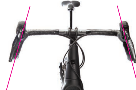
Brake hoods in line with the drop sweep
