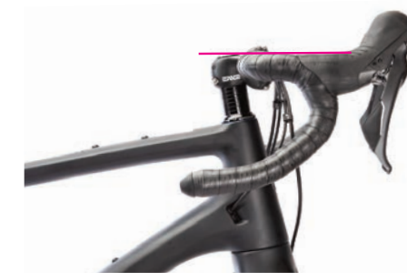
Brake hoods level (smooth transition) with handlebar
