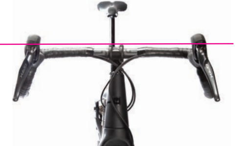
Brake hoods level with each other and level with ground
