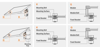
When using this kit with another brand of panel, you may need to change the module bolts to suit the mounting holes on the panel.
