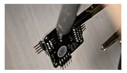
And that's everything!! Now you have a Naze 32 with all the inputs and outputs that you should need, the ESC's/Motor output and the R/C input are mandatory; on the other hand, you can decide of you want to install the Bluetooth/Telemetry pin set or the Battery/Buzzer alarm pin set.
