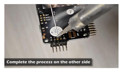
The next step is to solder the Buzz alarm/Battery voltage pin header. Apply flux on the pin holes.
