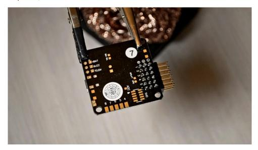
Now let's install the R/C input pin header. Apply more flux.
