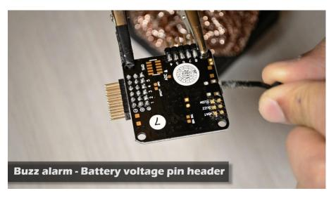
To solder this header, place it on the board and then apply some tin on the tip of your soldering iron and quickly apply the tin on one corner pin.
