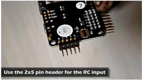
With this pin header we must use a similar technique as the previous one. Solder one of the lateral pins to make it stay in place, adjust if necessary.
