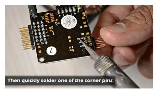
Check again that the pin header it's leveled and on the desired position. Then solder the rest of the pins.
