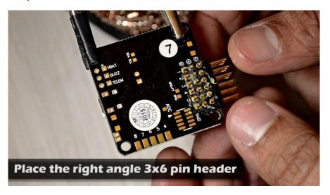
The trick to solder correctly this pin header is to solder one pin on one of the corners, in this case the top right corner, and then make the adjustments necessaries to have a leveled pin header in all the views.
