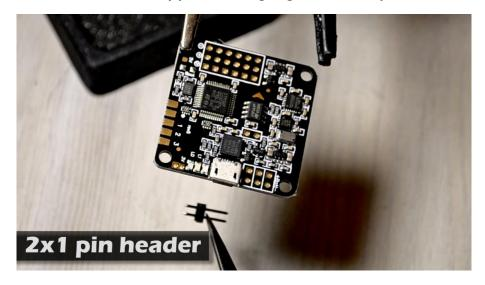
When soldering these pins, I strongly recommend you to use **soldering flux**. It helps the tin to flow faster and cleaner making the soldering process much easier.
