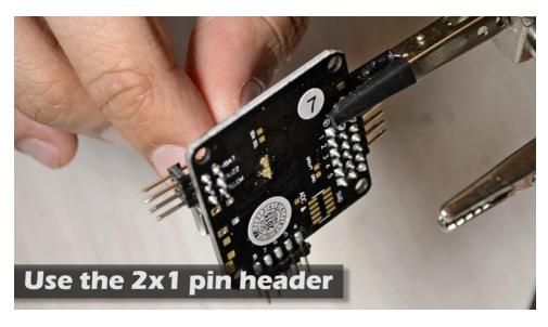
Finish the soldering with this small pin header.
