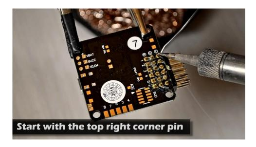
Once you have solder this pin check visually that the pins are straight and on the desired position, and then...
