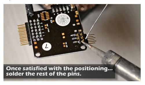
Finally, we are going to install the Bluetooth/Telemetry port. Apply some flux.
