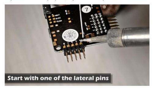
After you solder the first pin, flip the board and solder the opposite lateral pin.
