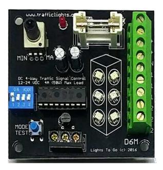
D6M - 4 Way Traffic Signal Control with 7 chaser control sequences
