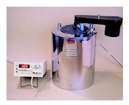
The Model CC01/M2A is the advanced version of the Model CC01/M2. With all the features being the same, The M2A model has the additional feature of being connected to a computer. It is supplied with an RS 232C interface to connect it to a computer with windows operating system. The M2A model automatically calculates the Calorific value of the sample.
