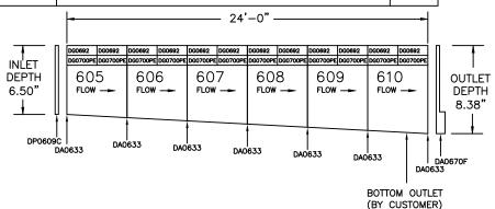
DRILL SIZE 3.50" FOR 3.0" SCH 40 & 80 PVC DRILL SIZE 4.25" FOR 4.0" SCR-35 SEWER & DRAIN DRILL SIZE 4.50" FOR 4.0" SCH 40 & 80 PVC
