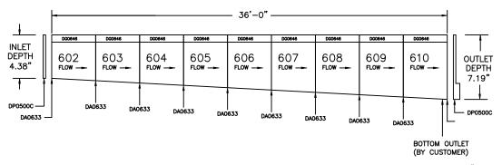
DRILL SIZE 3.50" FOR 3.0" SCH 40 & 80 PVC DRILL SIZE 4.25" FOR 4.0" SCR-35 SEWER & DRAIN DRILL SIZE 4.50" FOR 4.0" SCH 40 & 80 PVC
