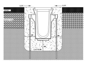
Set trench drain in channel surrounded by 4" of concrete with a minimum of 3,000 psi. Install #4 re-bar to stabilize drain while concrete is being poured. Make sure re-bar is 1" below finished surface.
