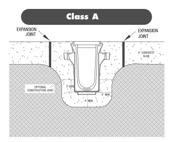
Set trench drain in channel surrounded by 4" of concrete or thickness of the concrete slab with a minimum of 2,500 psi.
