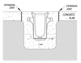
Set trench drain in channel surrounded by 4" of concrete or thickness of the concrete slab with a minimum of 3,000 psi.
