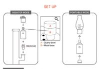
PORTABLE MODE Connect the Apollo base and atomizer to the bubbler. Also attach the silicone airflow regulator and sleeve from the bottom of Apollo base.
