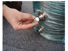
9. Now thread the nipple into the ball valve, ensuring that the valve's handle will face away from the tank once installed. Don't worry if you can't thread the nipple in very far by hand. Next install the ball valve / nipple assembly into the lower port on the tank. Again, thread it in as far as you can by
