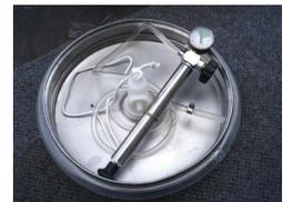
8. Now it is time to install the rest of the hardware. Locate your MoreWine! Hardware pack and confirm that it included a 1/2" stainless steel ball valve, nipple and plug. The nipple and plug should be pre-wrapped with teflon tape to ensure a good seal. Thread the plug into the upper of the two ports as far as you can by hand. If you have purchased a thermometer or thermowell to be installed in the tank, then install this instead of the plug.
