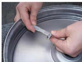
5. Now attach the tubing to the barb on the pump and secure it with the other hose clamp. This is a great time to make sure that everything is attached correctly and holding pressure. Loosen the black knob next to the gauge on the pump, and inflate the bladder until the pressure gauge is reading somewhere in the green zone. Note what pressure you inflated to, then set the lid aside for now. We'll want to come back in about 30 minutes to make sure no pressure has been lost.
