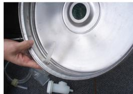
3. Now stretch the bladder the rest of the way around the lid's rim. The easiest way to do this is to set the lid vertically on the ground and hold it in place with your foot. Stretch the tubing up around the bottom of the lid with both hands so that the last portion to slide on to the rim is the part that is exactly across from the stem.
