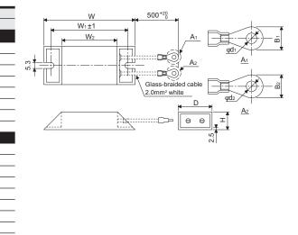
Notes: 1. For the 15K, connect the two supplied resistors (18 ohms) in parallel. 2. For the H15K, connect the two supplied resistors (18 ohms) in series.
