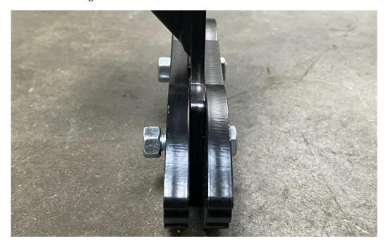
Attach the sleeves to the bar by fitting the tube through the holes on the outside of the bar, and secure it using the included button head bolts with a nut towards the inside of the bar.
