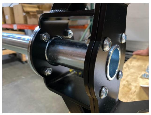
Attach the handles to the brackets by inserting them and aligning the holes in the bracket with the tapped hole in the handle and secure with a .75" bolt on each side, first using a washer on the outside of the bracket. While not necessary for the function, this washer will help preserve the finish in this area during repeated handle changing.
