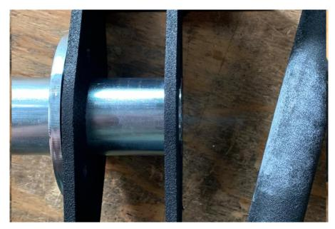
Using all the included bolts, place a washer on them and then insert them through all four holes on both sides with the threads oriented toward the middle of the bar. From there, add a washer to the other side and secure with a nut. Do not tighten beyond 23 lb-ft of torque.
