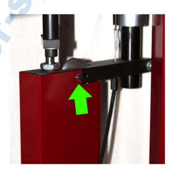
Thread the new cable through the grey shelf and around the two pulleys as shown.The end of the cable then slides into a slot in the end of the black steel bar.
