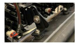
**CrossLink Supports.** These supports attach to a link, and are intended to stabilize the bar on longer windshield applications. If your kit includes one support, install it in the middle of the bar. If your kit includes two supports, space them evenly on the bar.
