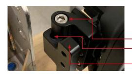
8. Loosely attach the end-mount base to the end mount connector, using the long M6 socket-head screw. Secure loosely, using a 5mm allen key. Note that the slotted section of the end-mount will allow for some adjustment of total length or curvature. Repeat for the other side. On one side, the long screw will be inserted from the top, and on the other, it will be inserted from the bottom.
