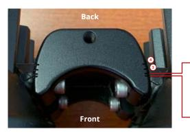
**Select Your Curvature.** The CrossLink technology allows you to build a straight or curved lightbar. Indicator markings are provided on each link and pod, to be used for reference.
