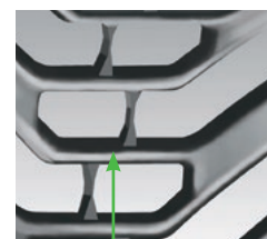
Nokian Forest King F tread depth measuring point beside tie-bar
