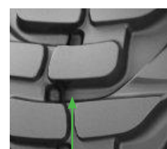
Nokian Forest King F2 tread depth measuring point beside tie-bar
