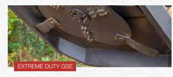
Intended Use: The Ground Shark™ Brush Cutter is designed for cutting brush and small trees up to 10" (178mm) in diameter while maintaining a 12" (305mm) maximum ground clearance. When equipped with the tooth kit, the attachment will also grind the remaining stumps down to ground level. Use in any other way is considered contrary to its intended use.
