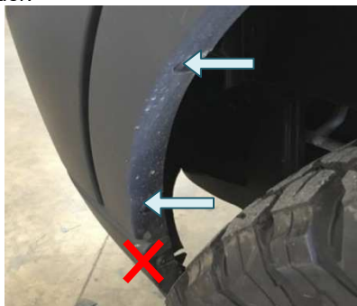
Figure 3: Fender Flare Plastic Rivets
