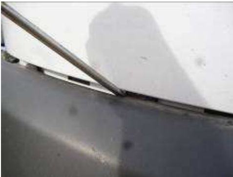
Figure 9: Prying Front Bumper from Grille
