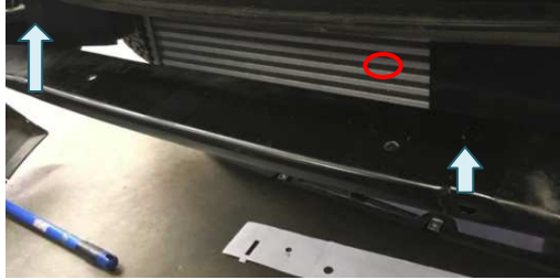
Figure 15: Holes Cut into Lower Sub-Frame
