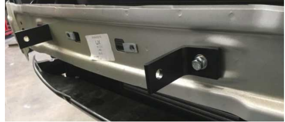
Figure 13: Attachment Brackets Attached to Sub-Frame
