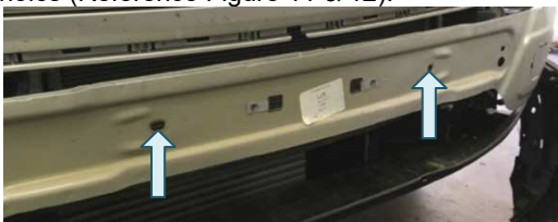
Figure 11: Holes to be Used for Installation
