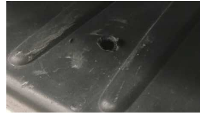
Figure 18: Hole Drilled Through Lower Plastic Stock Bumper
