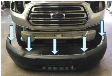
Figure 10: Front Bumper Removal
