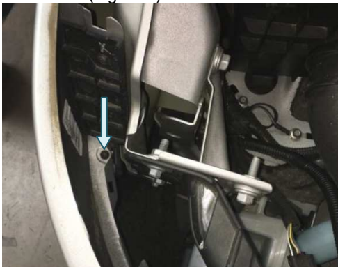
Figure 2: Bolts Underneath the Headlights
