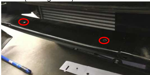
Figure 17: Holes Drilled Into Lower Sub-Frame
