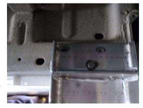
10. Once all of the Riv Nuts are installed you can bolt the nerf bar back to the vehicle.
