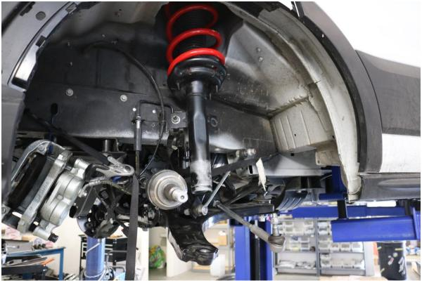
15) Remove the three upper strut nuts securing the strut to the chassis. Use a 15mm socket / wrench for removal (13mm for 2013-2017). On the driver (left hand) side of the vehicle, the nuts are accessible via the driver foot well.
