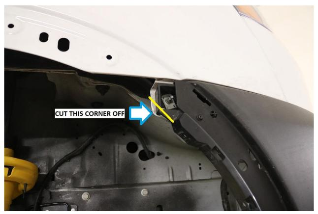
39) Lastly, the front bottom corner of the plastic front bumper fascia needs to be trimmed slightly for tire clearance.
