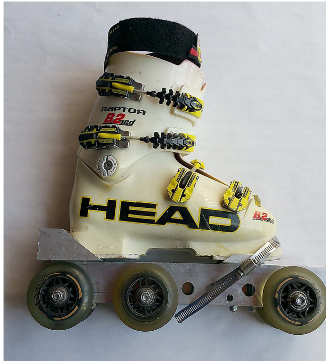
Outside of boot, axle nuts, screw and loose end of hose clamp
