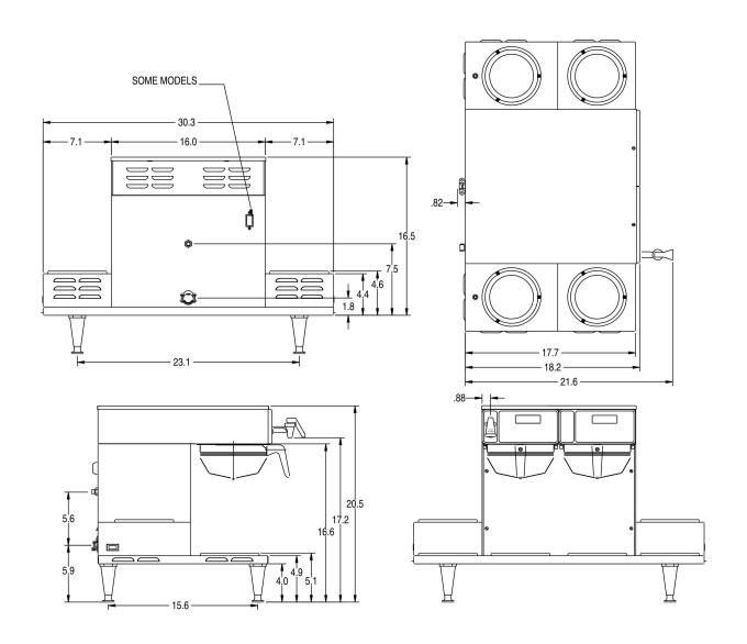
Electrical Configuration Option Volts-Factory Wired:120/208-240
