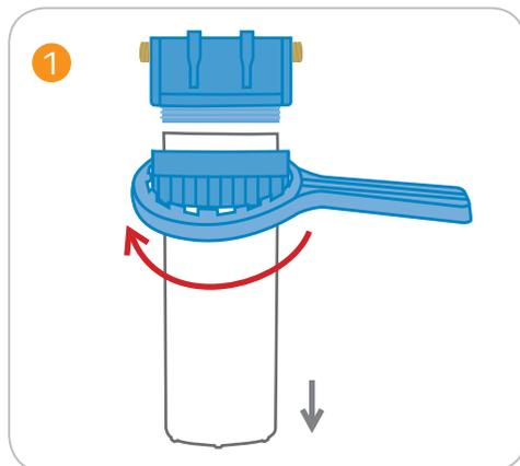
1 Unscrew the bottom part of the filter housing from the housing head using the housing key.
