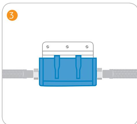
3 Attach the pre-assembled system to the wall and integrate it into the cold water pipe. To do this, connect the union nuts of the additional flexible connection hose to the angle valve and the inlet to the housing head (IN). Now connect the union nut of the loosened flexible hose (fitting) to the outlet of the housing head (OUT).
