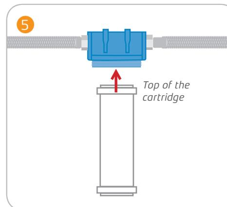
5 With its opening upwards, insert the cartridge into the housing head.
