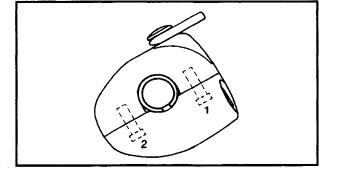
NOTE: \_\_\_\_\_\_ Tighten the screw 1 on the stop button side first. Then, tighten the other screw 2.
