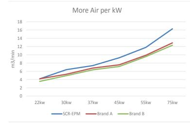
SCR's innovative high effciency airend has been oversized to ensure that air delivery is 10-15% higher than our competitors machines. The increased air delivery can allow users to select a lower powered EPM machine or use the additional flow to prevent assist compressors running at peak demand.
