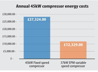
The above graph compares a 45kW fixed speed compressor running 6000 hrs per year with 2000 hrs per year off load running. SCR's 37kW 50EPM compressor produces the same flow as a 45kW compressor but for 18% less power.
