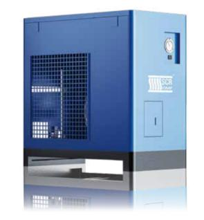
The high heat exchange efficiency design of the inlet and outlet temperature difference of 5  $^\circ$  reduces the demand of cooling capacity to a low level and achieves a high energy efficiency ratio. The stainless plate heat exchanger is used to prevent the dryer itself from becoming a source of pollution and to achieve high quality compressed air.
