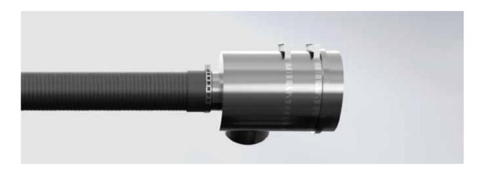
On the basis of the ordinary air filter, it adds a centrifugal separation structure design on the one hand, so that the air entering the air filter element is pre-separated to remove larger particles of dust, thereby effectively extending the service life and maintenance cycle of the filter element.
