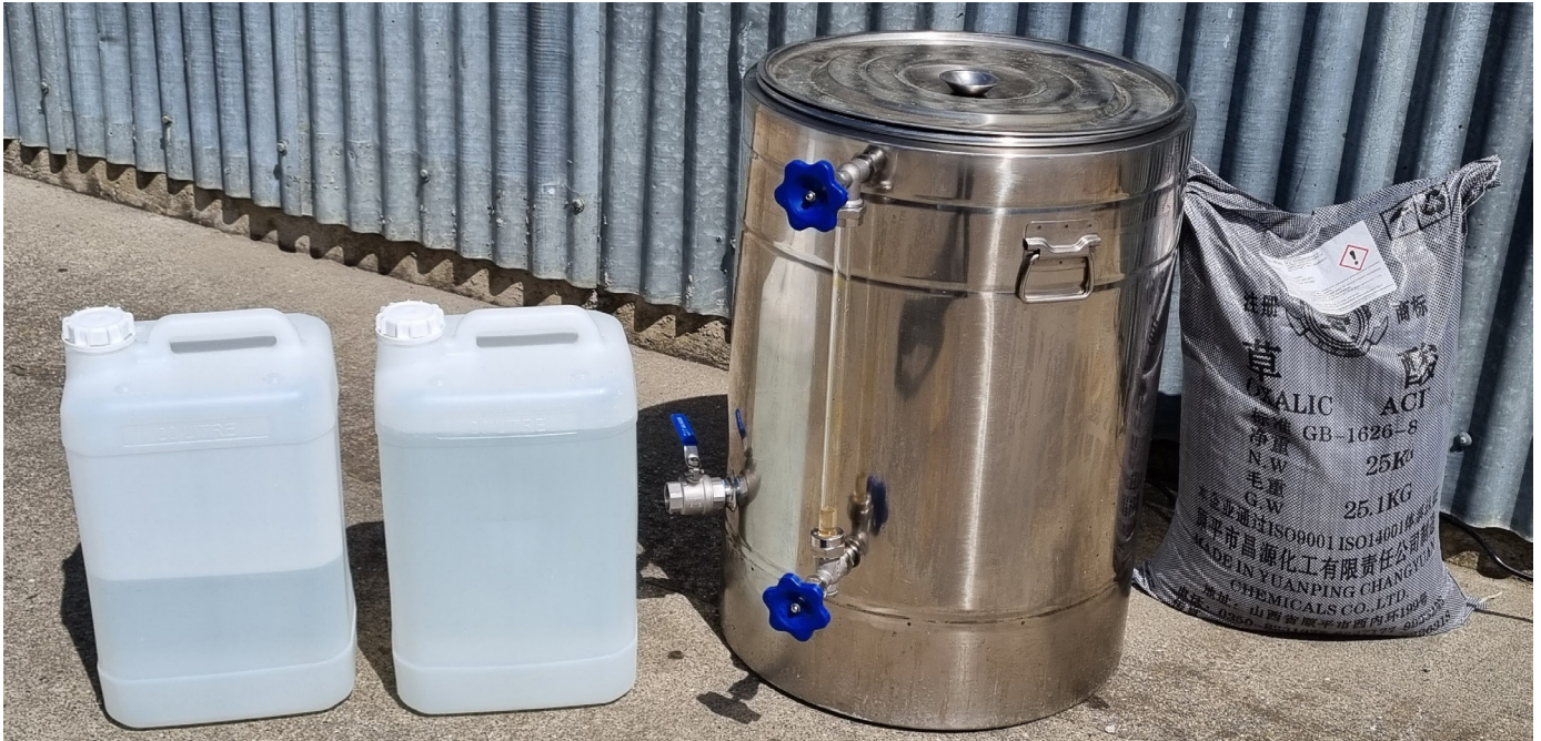
As shown above, 37.5kg (1.5 Jerry Cans) of Glycerine works great with a 25kg bag of Oxalic Acid as a starting point.
