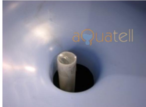
Once all of the resin has been added it is [very important to remove the piece of tape](#) from the top of the riser tube.
