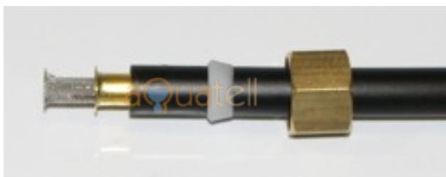
The brass tube insert and woven metal insert must both be pushed fully into the brine line. Once all the pieces have been attached to the brine line push it into the brine line adapter on the valve, and tighten down the brass nut to hold it in place. After completing this make sure that during the process of attaching the brine line to the valve, that the brine tank connection did not loosen.
