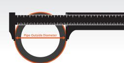
or centimeters. Record the diameter of the pipe in inches (centimeter measurements can be converted to inches by dividing by 2.54).
