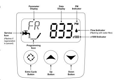
3. Press the Extra Cycle button. Use this display to adjust the Regeneration Time. This option setting is identified by "RT" in the upper left hand corner of the screen.
