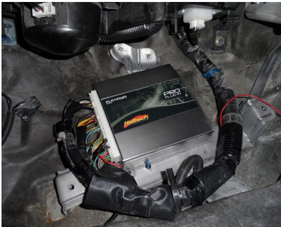
Figure 4 – Haltech ECU Mounted to Factory ECU Mount
