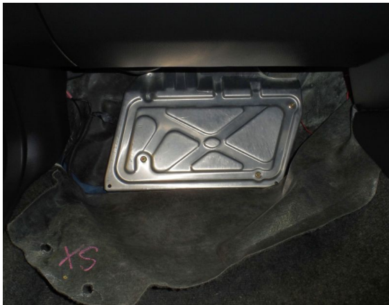
Figure 2 – ECU Protection panel under the carpet
