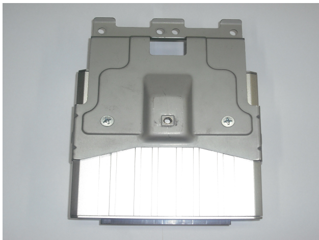
Figure 5 – Haltech ECU with original mounting bracket fitted
