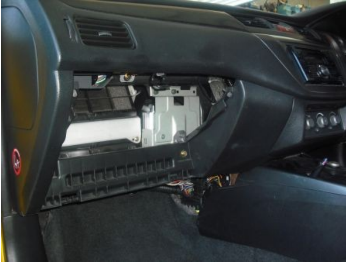
Figure 6 – Haltech Pro Plug-in ECU Installed
