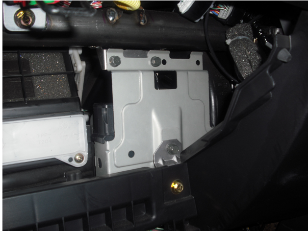
Figure 4 – OEM ECU in Original Mounting Position
