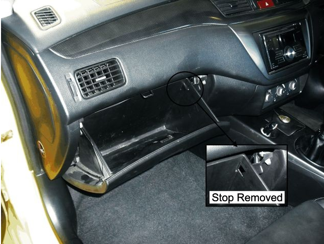
Figure 2 – Glove Compartment Removal
