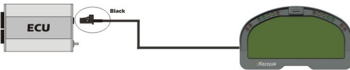
Figure 8 – Haltech ECU connected to a Racepak Dash
