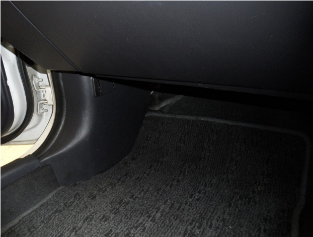
Figure 6 – Kick panel Re-installed
