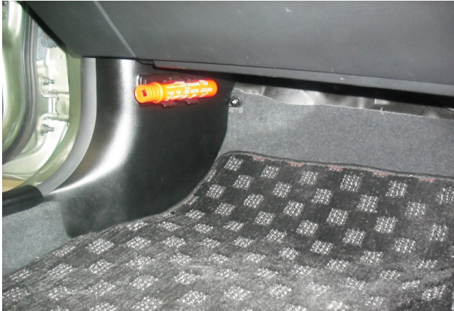
Figure 6 – Kick panel Re-installed
