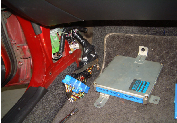
Figure 2 – Factory ECU disconnected and removed
