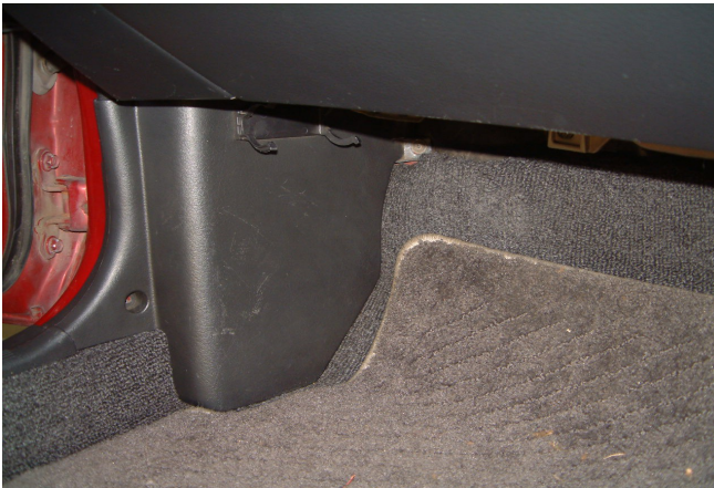
Figure 7 – Kick panel Re-installed
