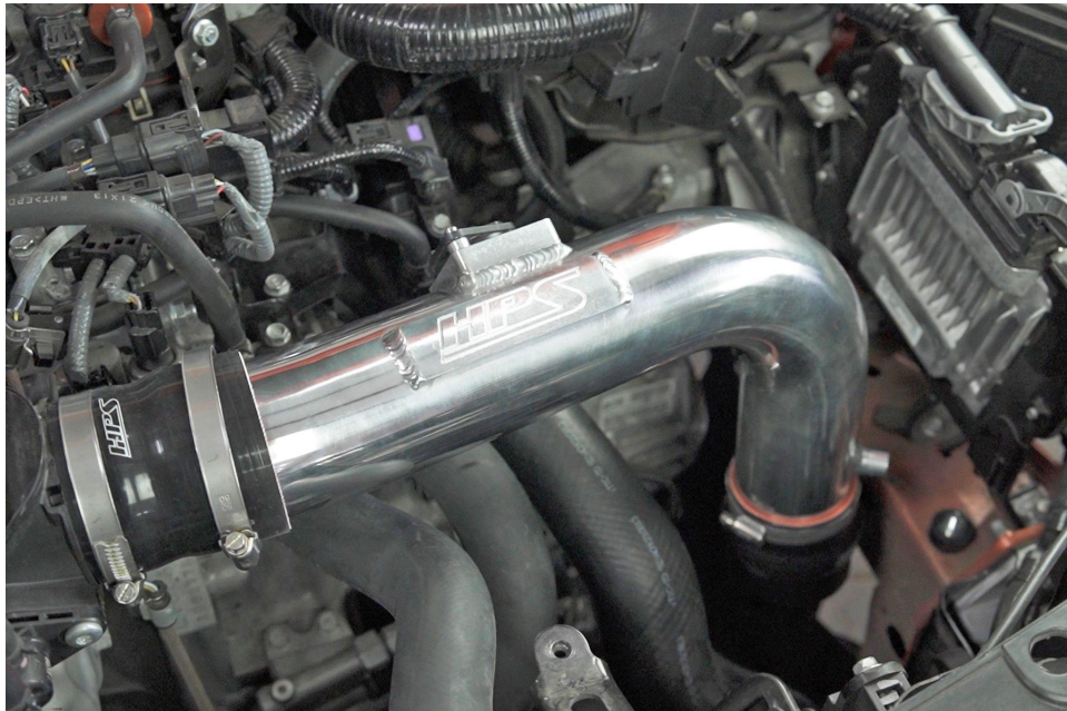
20. Insert the HPS intake pipe into the reducing coupler at the turbo inlet.
