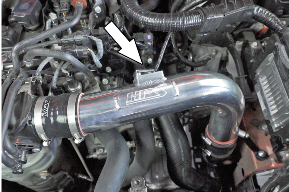
17. Reconnect the mass air flow sensor.
