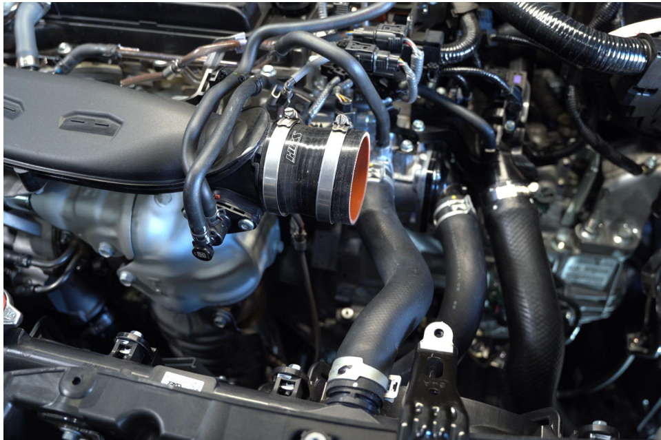
16. Install the reducing coupler along with the provided clamps onto the turbo inlet.
