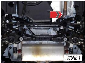
Cut the exhaust at the area located just after the welded joint, shown by the arrow in Figure 1.
