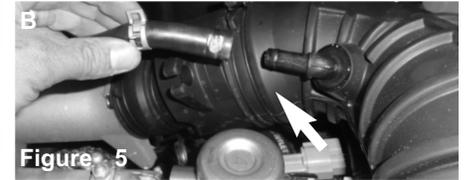
**Figure A:** Disconnect the recirculating diverter valve hose from the intake duct. **Figure B:** Disconnect the crank case and vacuum line.
