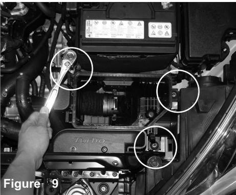
Use a 10mm socket, ratchet and extension to remove the three 10mm bolts on the lower air box assembly indicated by the arrow. Save 1 bolt for later install.
