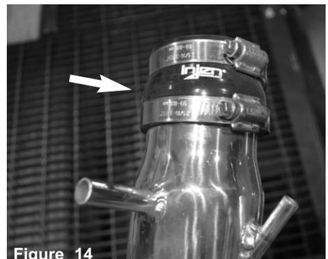
Install the step hose with clamps to the intake tube.
