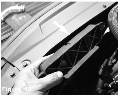
Loosen the 2 bolts holding in the front scoop vent and remove. Save 1 screw for later install.
