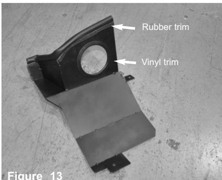
Install the provided rubber trim seal to the top of the heatshield and the vinyl trim to the hole on heatshield
